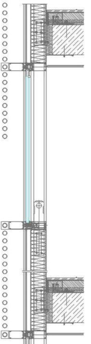
Figure 16 Detail façade showing integrated supply and hydrogen piping.
