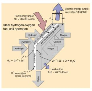
Figure 7 The diagram shows the chemical reaction that produces the electric current. [ThinkQuest New York City]
